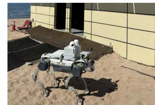
Deep Robotics' Jueying X30 robot dog for fully automatic outdoor inspection 雲深處絕影 X30 機器狗全自動戶外巡檢
