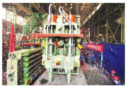
Producing slabs with max. thickness of 400mm. (from 300mm.) and increase production capacity of slabs by 1 mmt. p.a.(to 3.6mmt.)
